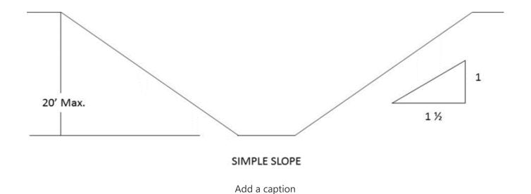
All excavations 20 feet or less in depth which have vertically sided lower portions shall be shielded or supported to a height at least 18 inches above the top of the vertical side. All such excavations shall have a maximum allowable slope of  $1\frac{1}{2}$ :1:
