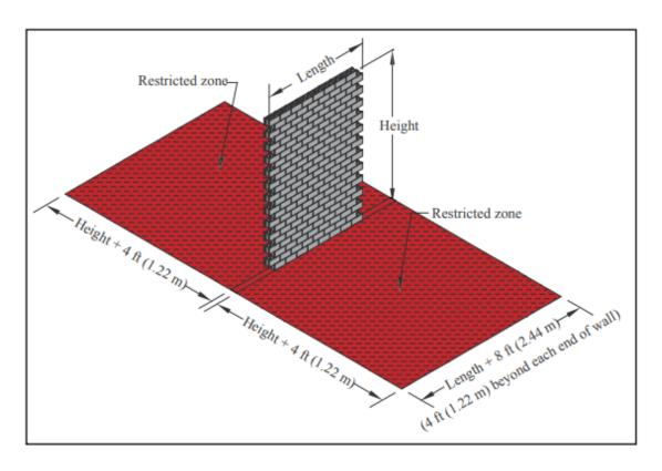
■ Figure 1-Restricted Zone for Masonry Walls
