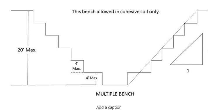
c) All excavations 20 feet or less in depth which have vertically sided lower portions shall be shielded or supported to a height at least 18 inches above the top of the vertical side. All such excavations shall have a maximum allowable slope of 1:1:
