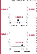
WHEN LIFTING VERTICALLY, THE LOAD WILL BE SHARED EQUALLY IF THE SLING 2 CENTER OF GRAVITY IS PLACED EQUALLY BETWEEN THE PICK POINTS.IF THE WEIGHT OF LOAD IS 10.000 KG, THEN EACH SLING WILL HAVE A LOAD OF 5.000KG AND EACH SHACKLE AND EYEBOLT WILL ALSO HAVE A LOAD OF 5.000 KG
