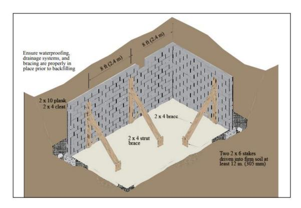
Figure 3-Typical Temporary Bracing for Concrete Masonry Basement Walls (ref. 6)
