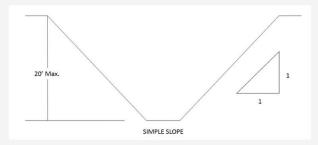
b) All benched excavations 20 feet or less in depth shall have a maximum allowable slope of 1:1 and maximum bench dimensions as follows:
