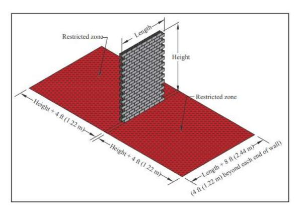
■ Figure 1-Restricted Zone for Masonry Walls
