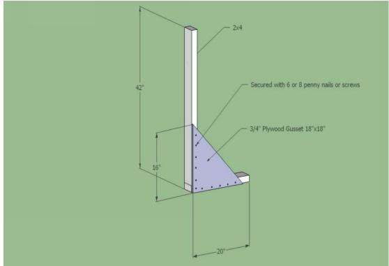
Wood Guardrail Construction Guide Section 36: Fall Protection
