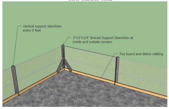
Steel columns should be punched to support guardrails. Concrete columns may have pvc block outs installed to support the cables.
